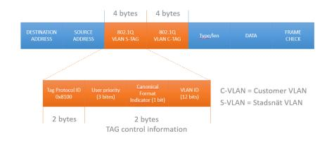
Picture: Specification of VLAN-tag function for Ethernet Medium
