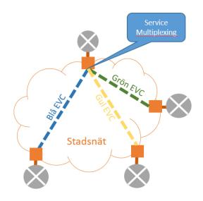
The figure shows three EVC:s, established through a joint transfer point. The EVC:s multiplexes based on VLAN. This equals solution 2, E-line EVLP and is preferred to the buyer.
